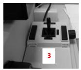
Motorized stage joystick and focus knob
